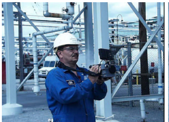
Figure 1. Because the moisture density gauge must contact the surface of the insulation, the use of a man-lift is required for pipe inspection. IR works great from ground level.
