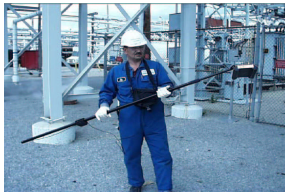
Figure 1. Because the moisture density gauge must contact the surface of the insulation, the use of a man-lift is required for pipe inspection. IR works great from ground level.
